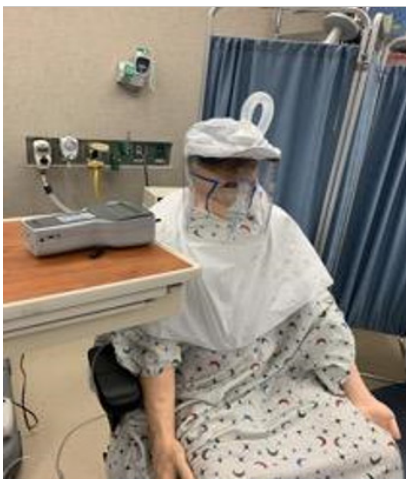
Figure 2 (Left) Particle count test set-up. (Right) Counts of 0.3 and 0.5 µm particles during 3 min of nebulising without the ARIEL (control) and with the ARIEL. ARIEL, Aerosol Elimination Device
