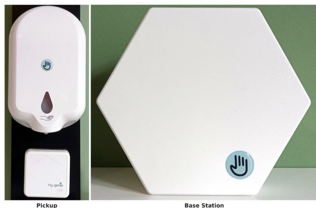
Figure 1 Components of Hy-genie Lite. Pickup sensors are small battery-powered devices that are mounted beneath soap or gel dispensers and use capacitance sensing to detect operation of the dispenser. When usage of the dispenser is detected, a time stamped message is sent to a central server via the nearest base station. The base stations act as routers for the messages sent by pickup sensors. Data stored in the base station are then visible on a computer dashboard. The daily counts of the number of uses of each dispenser, as represented by the counts of the number of sensor messages, were analysed during this study.
