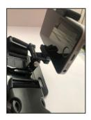
Side view - smartphone attached to the harness (screen should face the wearer).
