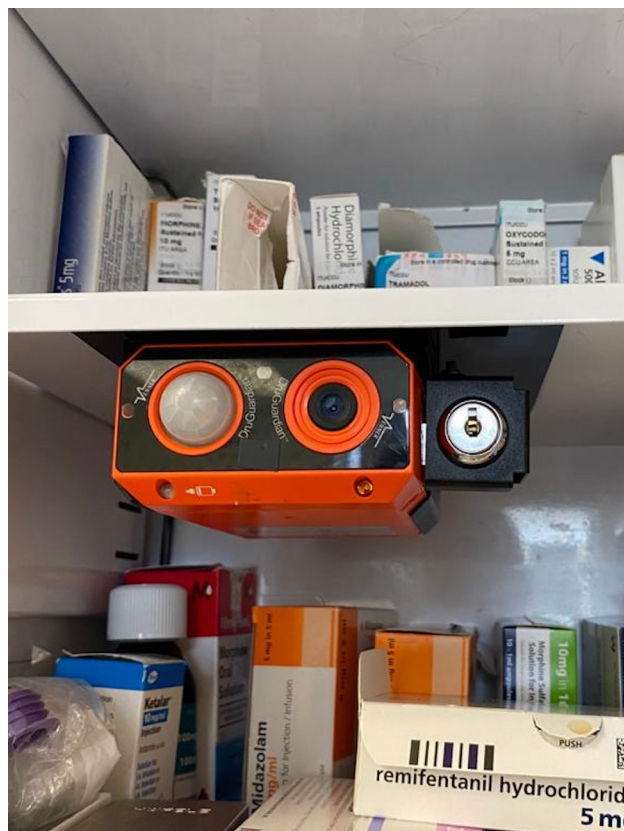
Figure 1 The DruGuardian device, demonstrating the camera, motion detector and light detector.
