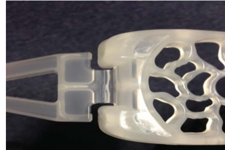
Figure 13 The redesigned shorter hinge. The sharp edges of the folded living hinge are now recessed behind extensions to the platform. Once folded for use, each arm has two pedicles lateral to the hinge that rest over the outer edges of the platform. As soon as the hinge starts to 'give' with pressure, these pedicles push tight against the platform thus ensuring strength and stability.
