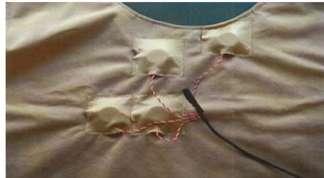
Figure 2 Placement of the speakers in standardised manner. Each speaker is attached to a different sound from the multitrack player.
