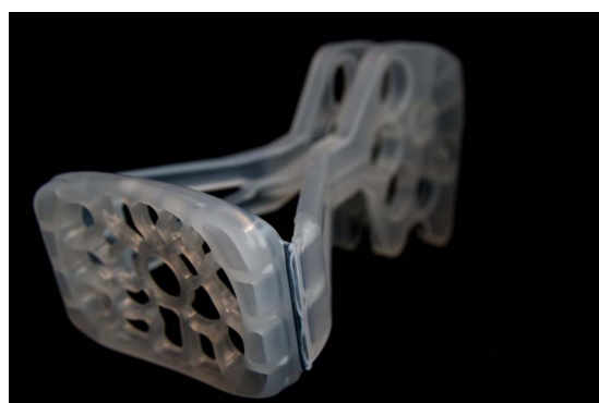
Figure 12 The initial hinge design—strong but with a sharp leading edge that could result in trauma on insertion.
