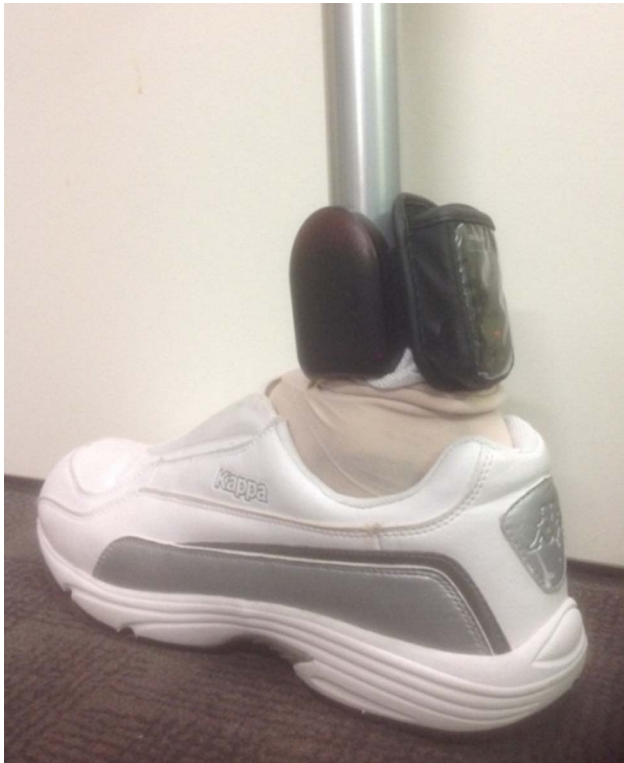
Figure 1 The StepWatch3 Activity Monitor (SAM) and global positioning system device were attached to a prosthesis. The SAM was attached according to the manufacturer's recommendations of positioning the device slightly above the position of the lateral malleolus.
