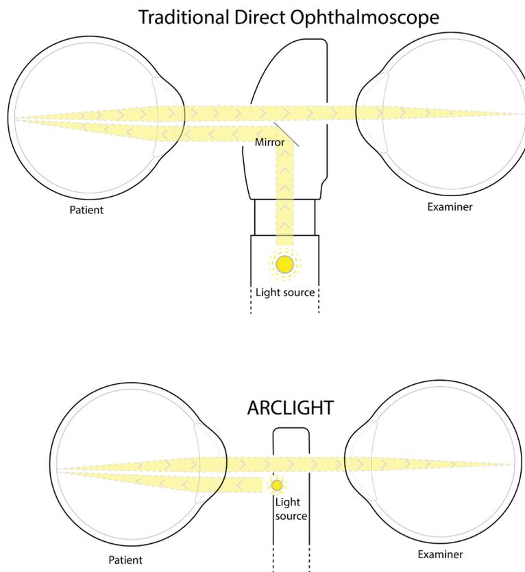
**Figure 2** The Arlight illumination uses a light emitting diode placed directly below the viewing hole, facing the patient, creating a near-axial light source unlike the traditional direct ophthalmoscope, which uses a mirror to redirect light into an axial path.
