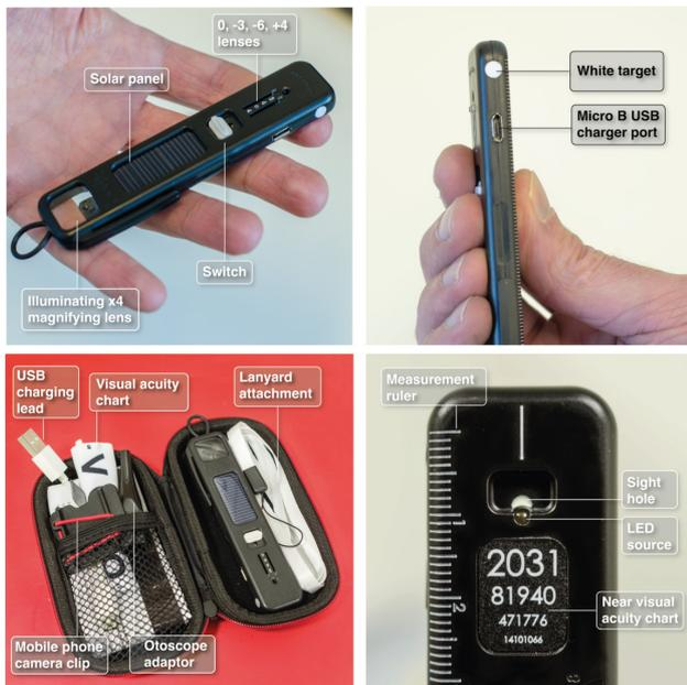
**Figure 1** The Arlight with selected features highlighted.
