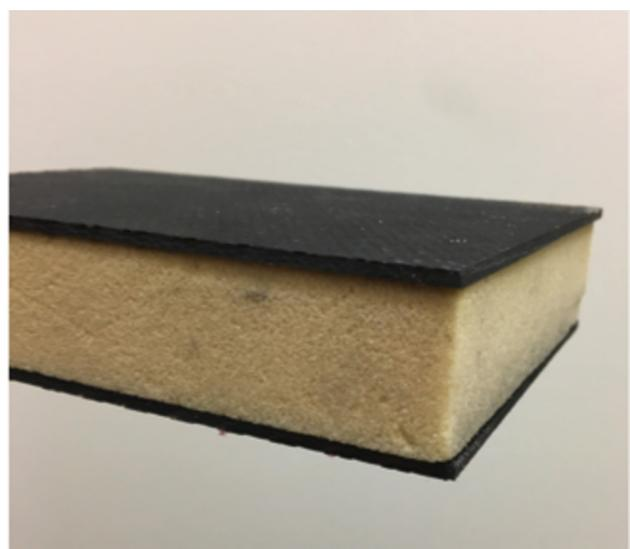
**Figure 3** Sawbone core with carbon fibre lining.
