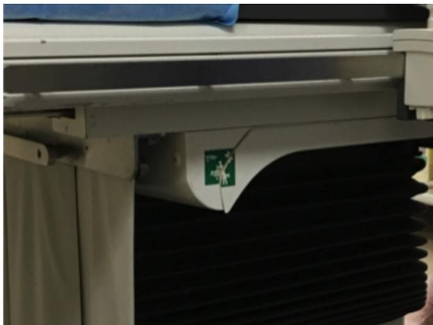
**Figure 1** Crack in the base attachment to an existing table.
